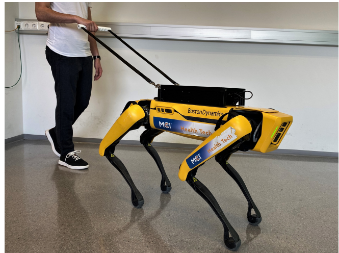
Fig. 5. The robot Spot with a dog leash to guide the blind or strong visually impaired person to the desired destination.
